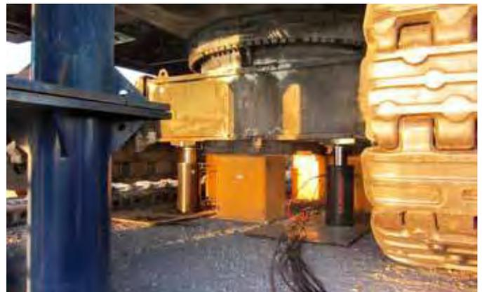
**THE *syncMASTER* MULTIPLE POINTS SYNCHRONOUS LIFT SYSTEM ALLOWS FOR UP TO 16 POWER PACKS TO BE CONTROLLED BY ONE MASTER UNIT, GIVING A MAXIMUM OF 128 INDIVIDUALLY CONTROLLED CYLINDER POINTS.**
