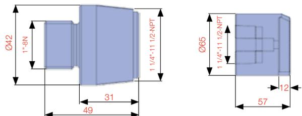
ZAM1245 and ZAM1246 allows Durapac RG 10 ton series cylinders (excluding RG-101) to be used with CRK-10 attachments.
