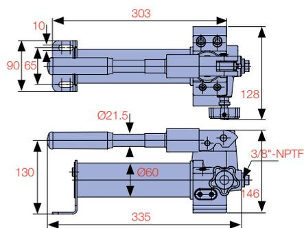
THE **P-SERIES** STEEL BODIED MANUAL HAND PUMP RANGE OFFERS A WIDE CHOICE OF TANK AND FLOW OPTIONS WHERE MANUAL PORTABLE HYDRAULIC POWER IS REQUIRED.
