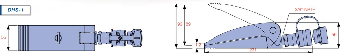
THE **DNS-SERIES** OF NUT SPLITTERS CONSISTS OF SEVEN MODELS FOR HANDLING DIFFICULT TO REMOVE NUTS RANGING FROM 10 - 75 MM A/F CAPACITY.
