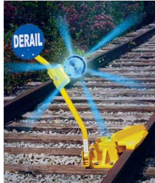
4115-01 Barricade-style, 7" diameter shatterproof Lexan lens, uses two 6-volt batteries. Battery case bolts to light-bracket. On-off switch and photo-electric cell. Flashes 60 times/min. Weight 3 lbs. Other lens colors available.
