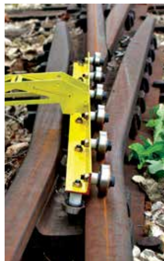
Two-piece assembly features spring-loaded piston for precise gauging.
