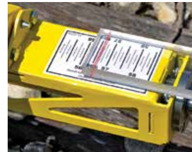
Gauge scale (55.5 - 58.5") can be read through a lexan lens from either side of Roadmaster.
