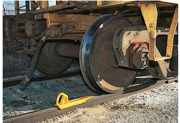
Replace skids when tongues become deformed. Skid tongue must lie dead flat on the rail to be effective.
